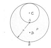
(a) A solid non-conducting sphere of radius a is filled with positive charge of uniform charge density  $\rho$ . Then a smaller sphere of radius  $\frac{a}{2}$  is carved out as shown in the figure and left empty. What are the direction and magnitude of the electric field  $\mathbf{E}$  at A? At B?
